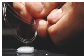
Researchers grow a brown, light-absorbing material for the solar generators on optical fiber (courtesy Gary Meek, Georgia Tech).
